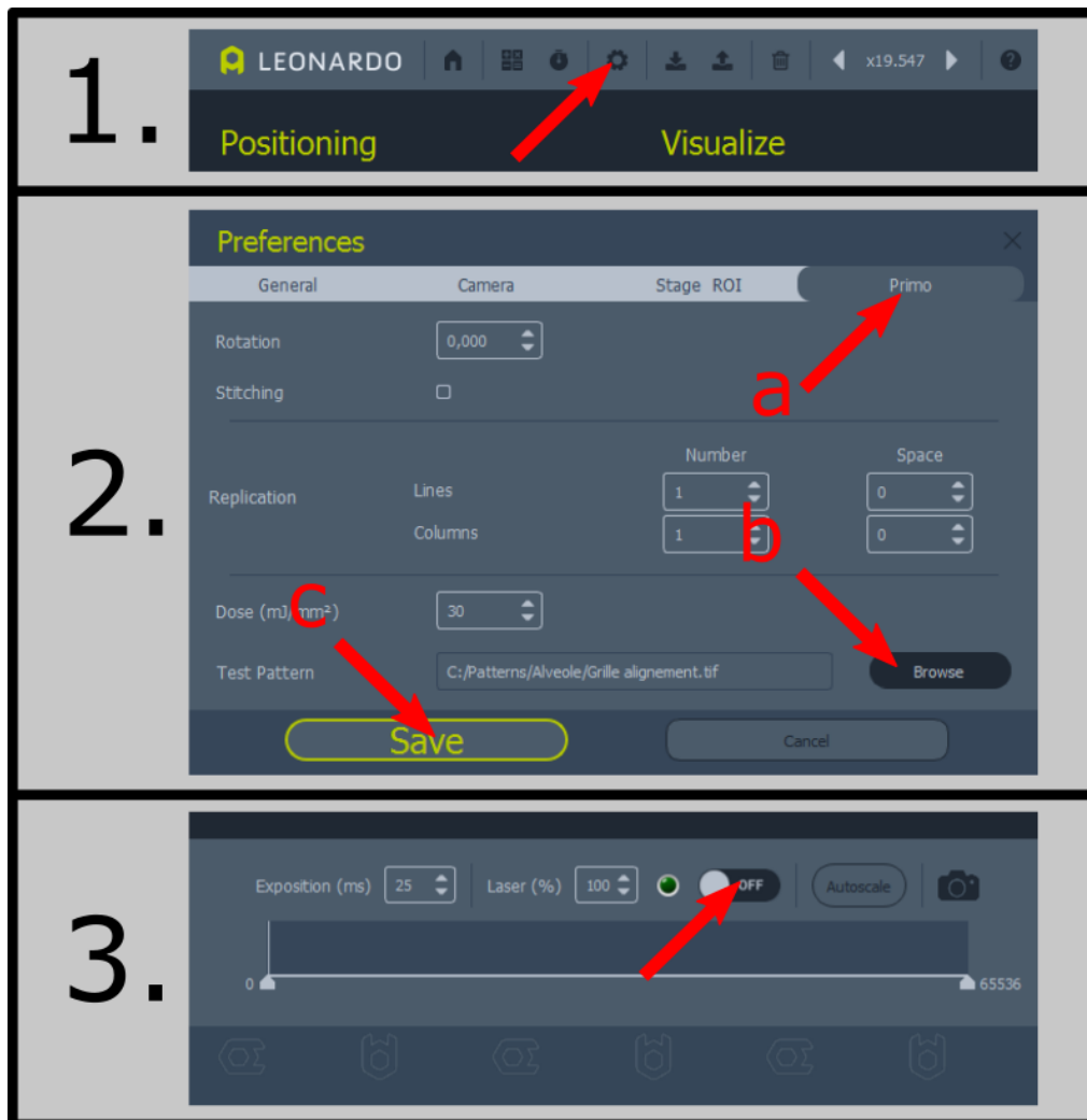
Figure 4: Using continuous mode with Leonardo: 1. Open “preferences” menu in top left corner of Leonardo software. 2. Go in the “Primo” tab (a) and choose your pattern using the Browse button (b) then save your choice with the Save button (c). 3. Start illumination by clicking the ON/OFF button, the chosen pattern will be projected where the camera is looking at. Use the same button to turn off the UV illumination.
