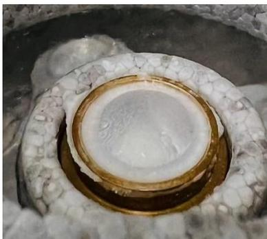
4. Replace the filter papers on the blotting pad whenever necessary. e.g. after blocking a maximum of 16 grids, or the filter paper is too humid after being inside 100% humidity chamber for a long time.
