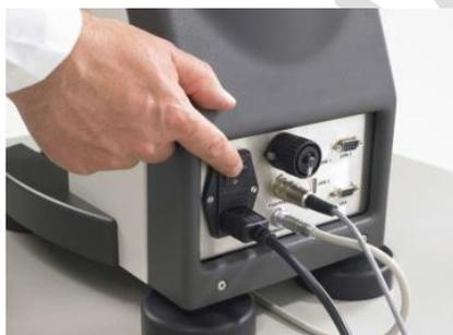
**Note: If the Vitrobot is not turned off with the switch at the back, the system WILL come back online after a while and stay on! Please make sure you double check!**
