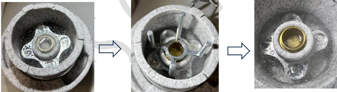
3. Excess ethane in the central cup (a meniscus appears outside the horizontal plane of the cup) may be removed with some filter paper.
